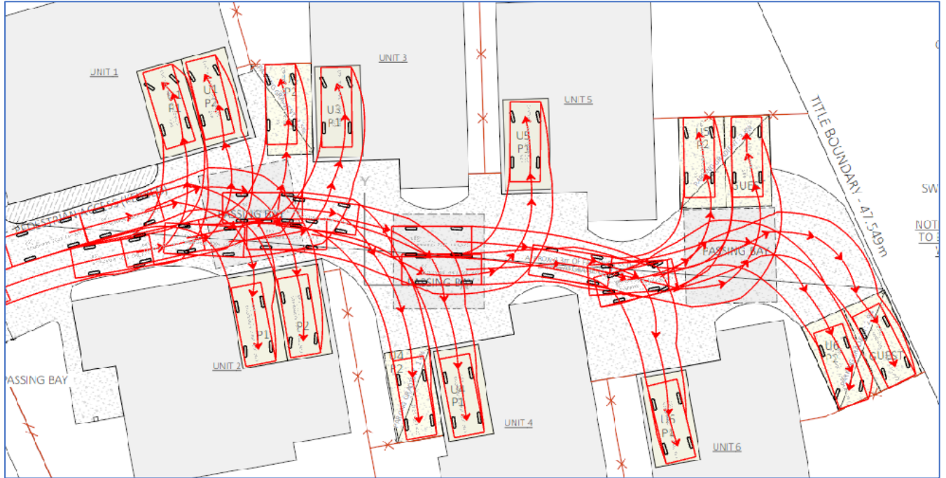
B85 vehicles entering the parking spaces
