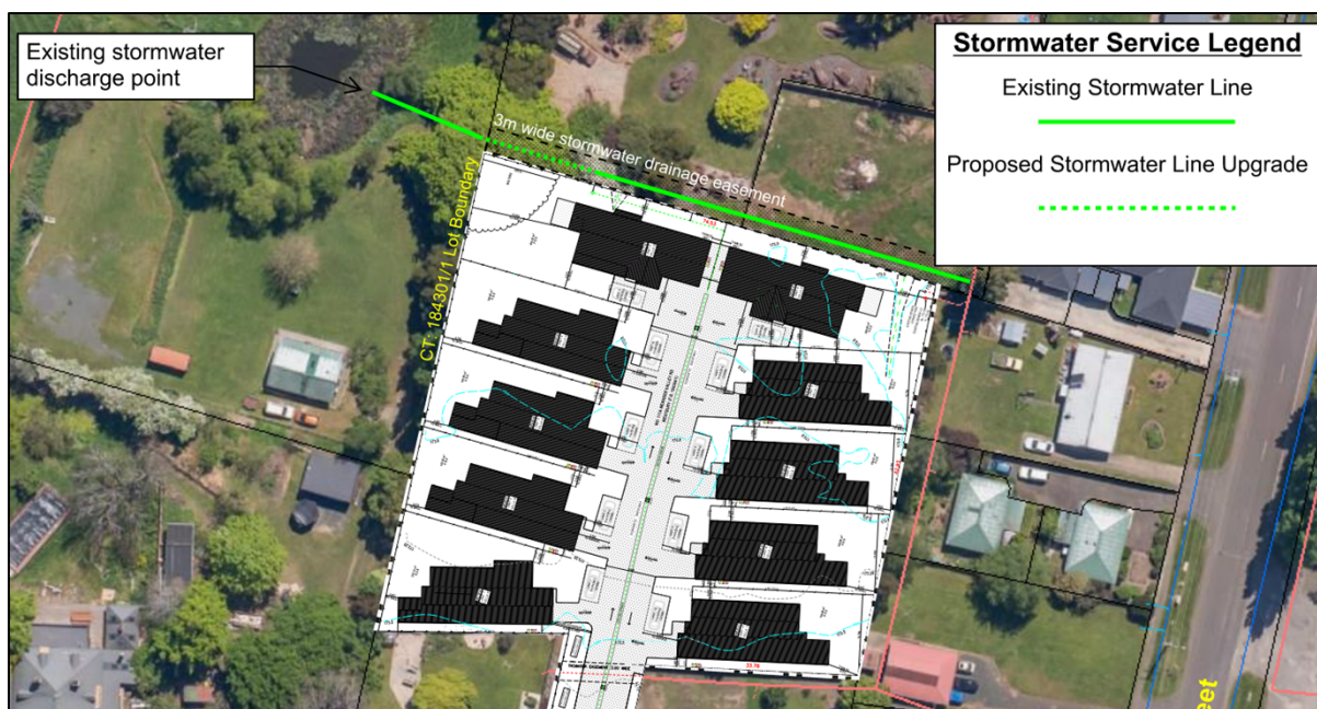
Figure 4 - aerial image illustrating the location of the proposed stormwater upgrades within the context of the proposed development and adjoining lots.
