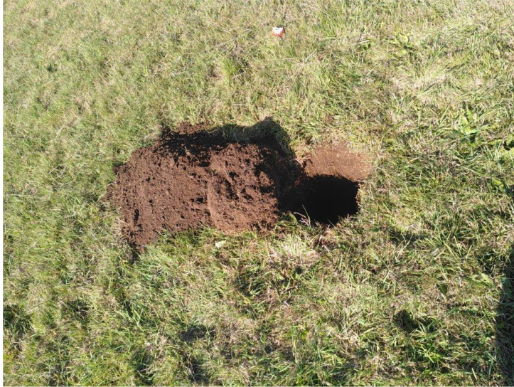
Photo of Test hole
